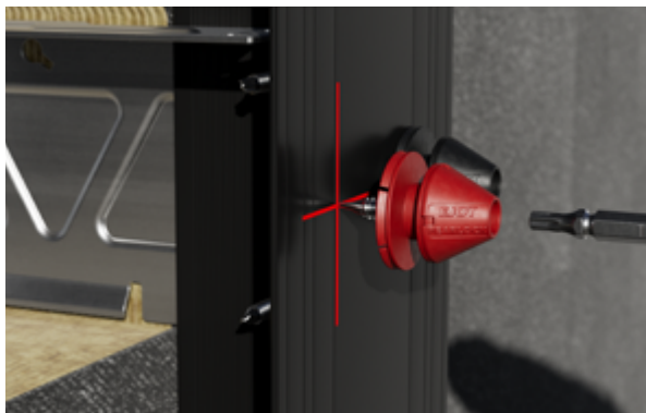
Position the PEARLOCK® system on the aluminium or steel substructure and fasten it with LT-TD screws using the extended TX25x70 bit.
