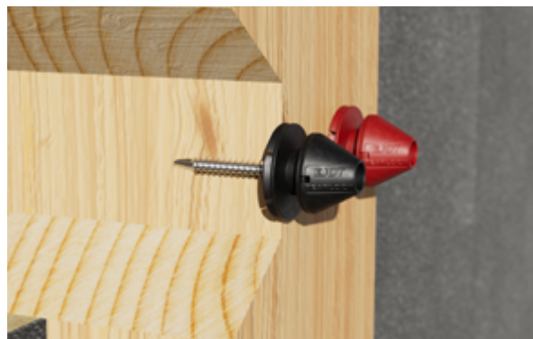
The fixed-point variant (red) completely surrounds the screw's stop collar, preventing relative movement between the components. It provides a reliable fastening of the cladding. The sliding-point variant (black) also engages the stop collar and centres it by means of a ring connected by four fine retaining bars. Under transverse loads, such as those caused by thermal expansion, these bars are designed to break away, allowing controlled movement of up to 3 mm in any direction.
