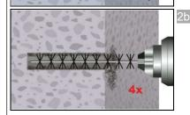
Attach brush RBT according to Table B3 to a drilling machine or a cordless screwdriver. Brush the bore hole minimum 4x over the entire embedment depth in a twisting motion. (If necessary, a brush extension RBL shall be used.)
