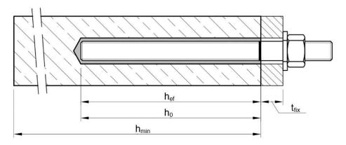
$t_{fix}$  = thickness of fixture
