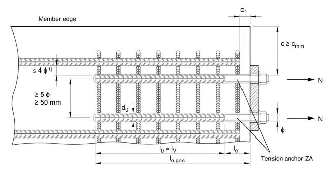
If the clear distance between lapped bars exceeds 4φ, then the lap length shall be increased by the difference between the clear bar distance and 4φ.
