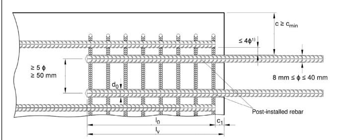
If the clear distance between lapped bars exceeds 4φ, then the lap length shall be increased by the difference between the clear bar distance and 4φ.
