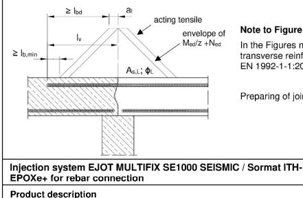
Installed condition and examples of use for rebars
