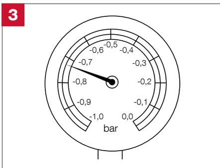
Provided the suction pressure remains constant, the assembly is then air- and watertight.
