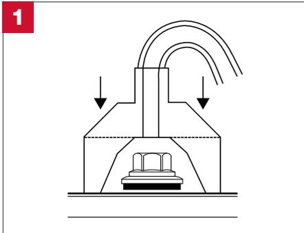
Put the nosepiece over the fastener and apply slight pressure ensuring that an initial seal will be obtained. Ensure a smooth and airtight surface.
